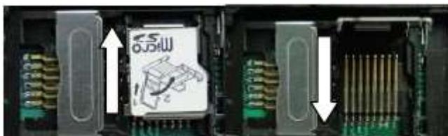
**5.1.3** Insert the Standard SIM card into the SIM card holder tray. Please note that Micro and Nano SIM cards are not supported.
