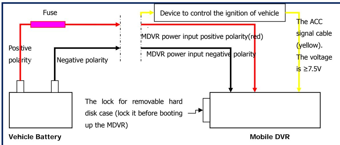
1. The MDVR cannot be installed on the vehicle floor directly. MDVR housing must be insulated with the body of the vehicle. External protection cap or box is necessary for waterproof and dustproof.
