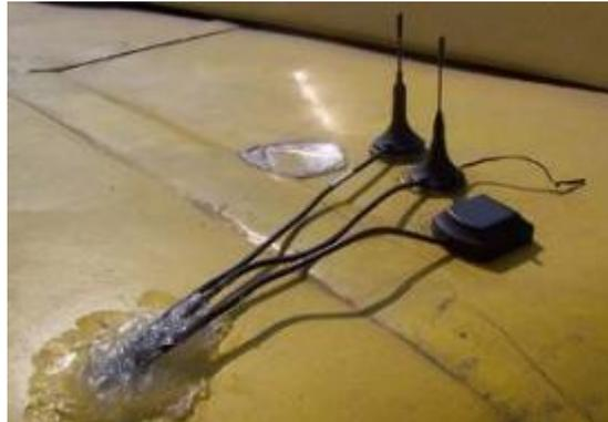
If drilling hole is not allowed by bus company or bus operator, then please install the antenna just inside of the vehicle
