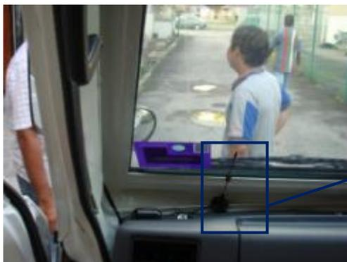
The WIFI antenna near dash mounted panel in bus
