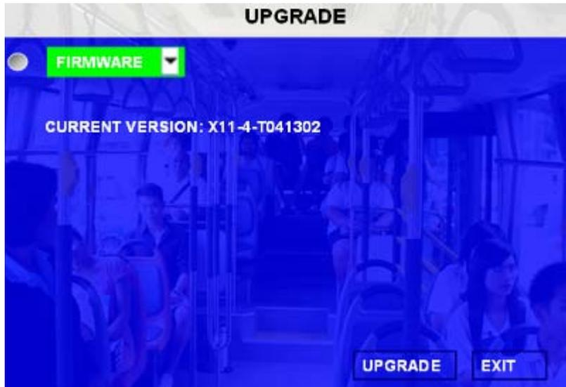
Please do not disconnect the power supply for MDVR or remove the thumb drive during firmware upgrade.
