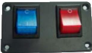
Generally the alarm system for driver is installed close to him for easy operation. The signal from MDVR to front part driver panic button connected with 3\*0.2 wires.
