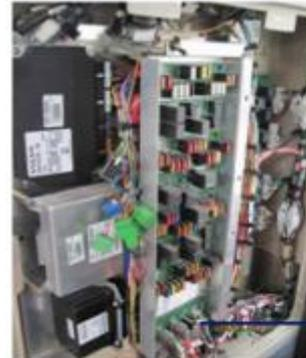
Get the power from the control box. Connect with the MDVR by fuse->
