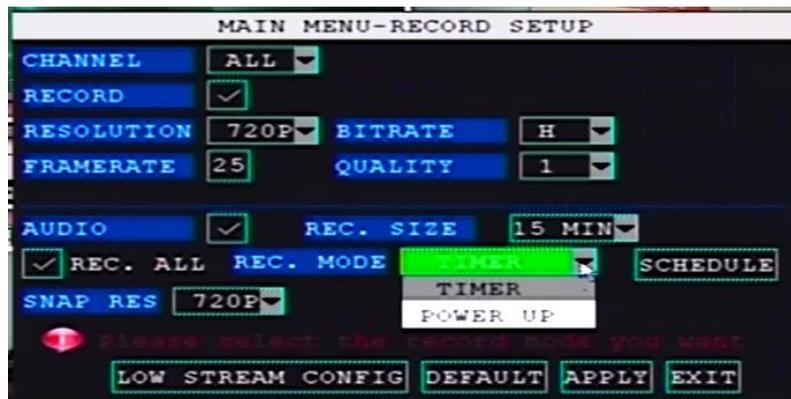
System allows the single channel record configuration, also allows to set up the same configuration for all channels.
