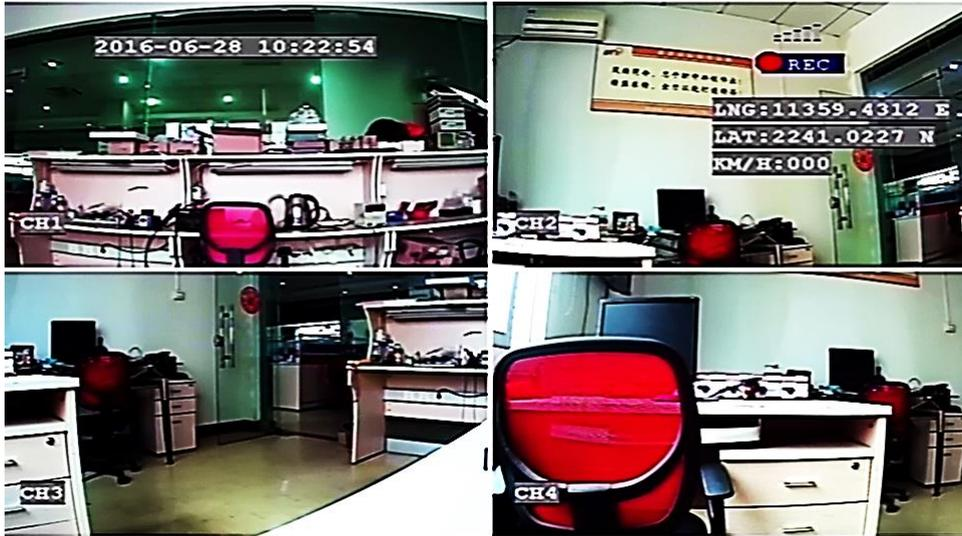
After the device power up, enter into the preview mode. The default interface is quad screen display, Users can configure display mode in the system menu, such as single channel preview or multi-channels preview.
