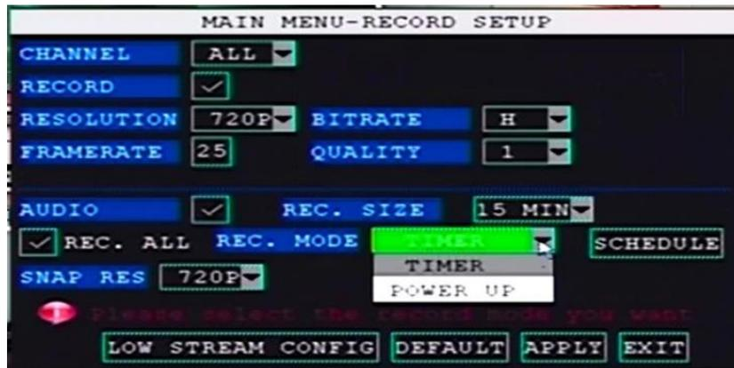
**Regular: As long as within the configured period and there are available storage devices, DVR will record, this mode does not support manually stop record.**
