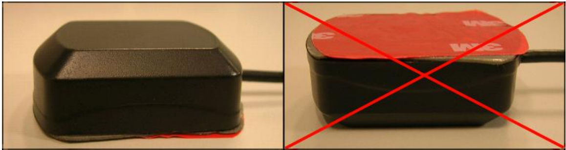
Figure 36 GPS antenna correct mounting.
